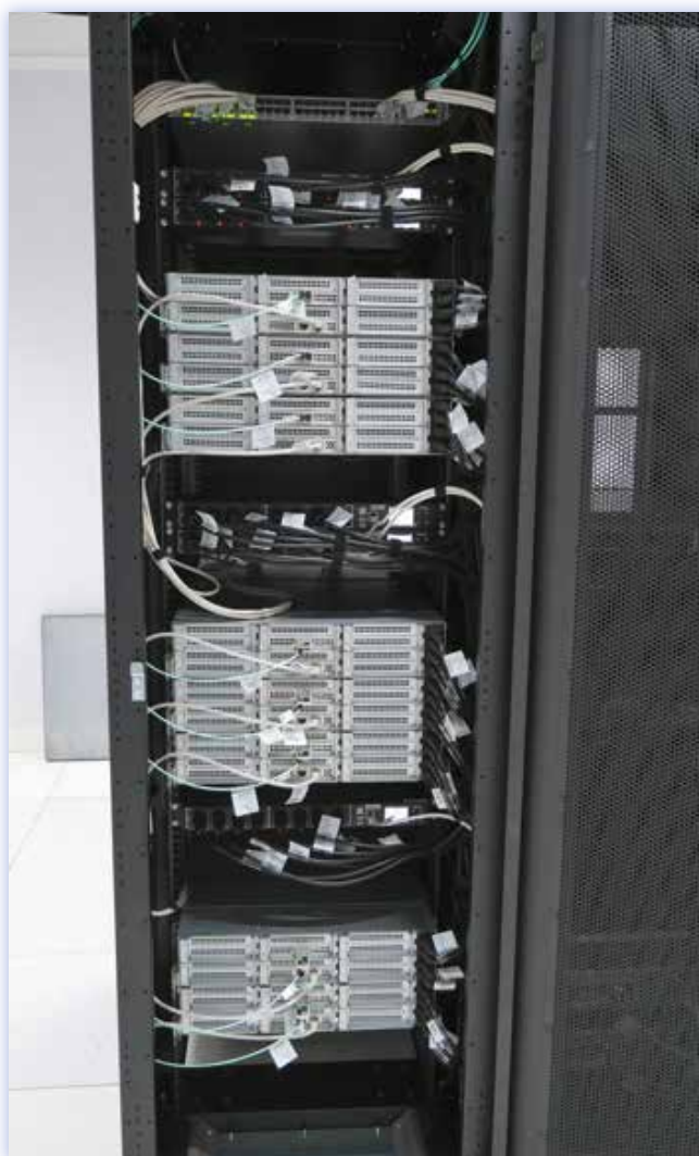
← Kelly , a scalar prototype based on the ARM architecture, deployed at CEA DAM.
